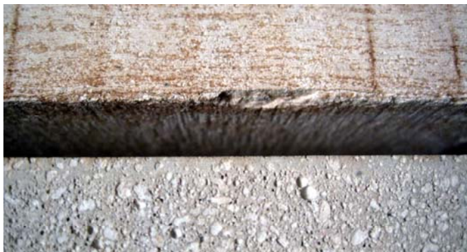
Wet material freezing (-28°C) and heating (+250°C) 1 cycle: glass fibre reinforced concrete (below) limestone fire protection boards (above) showing splitting
