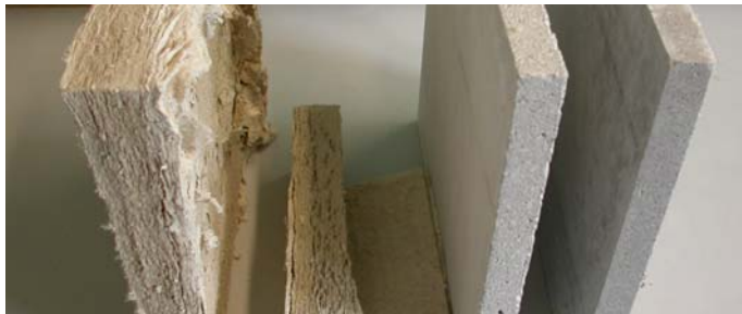
Wet material freezing test after 100 cycles: limestone fire protection boards (left) glass fibre reinforced concrete (right)
